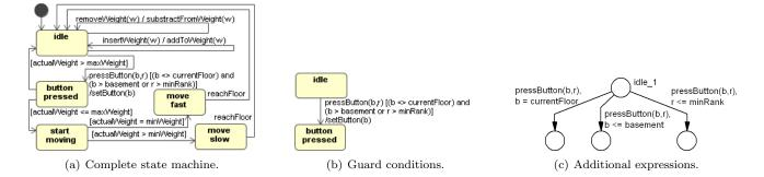
Figure 1: Model of a freight elevator control.
